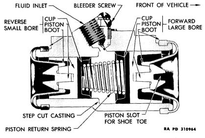
Figure 14 – Step-bore Wheel Cylinder with Slotted-insert Type Piston
