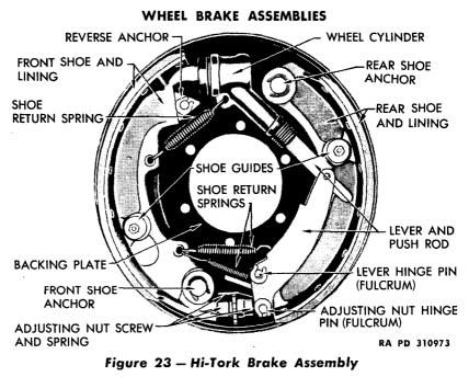
of the brake assembly. These locating points are reversed on the front brake shoe. Eccentric anchor pins are used. The rear shoe is anchored in a fixed position at the heel end of the shoe, by an anchor pin located near the wheel cylinder.
