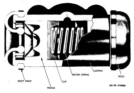
Figure 10 – Straight-bore Wheel Cylinder with Socket Type Piston
