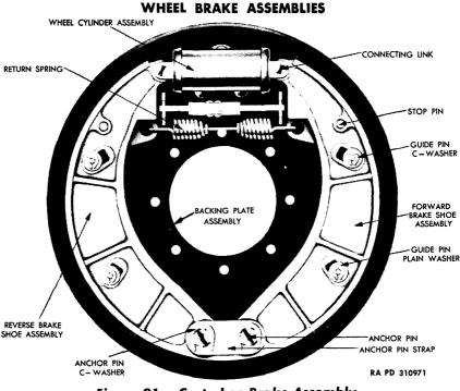
Figure 21 – Cast-shoe Brake Assembly
