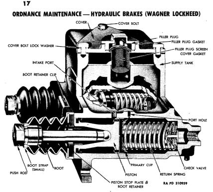
Figure 9 - Twin-bore Master Cylinder
