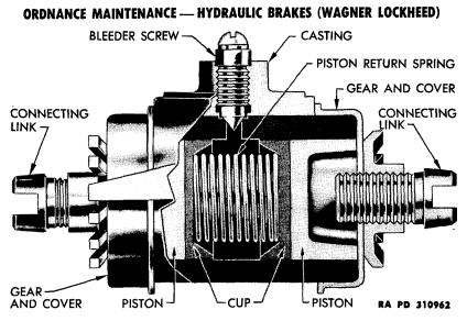
Figure 12 — Straight-bore Wheel Cylinder with Metal Boots
