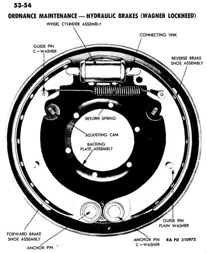
Figure 22 - T-section Brake Assembly
