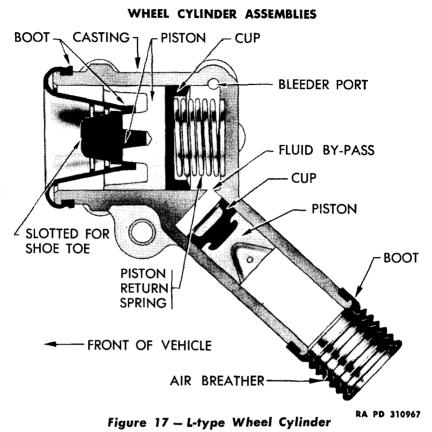
b. The L-type wheel cylinders are manufactured in the following diameters:  $1\frac{3}{8}$ - $1\frac{1}{16}$ -inch,  $1\frac{1}{2}$ - $\frac{3}{4}$ -inch,  $1\frac{3}{4}$ - $\frac{7}{8}$ -inch.
