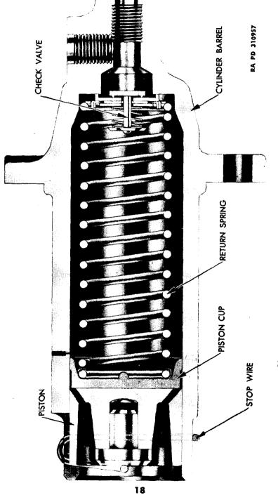
Figure 7 – Master Cylinder Head and Barrel Assembly
