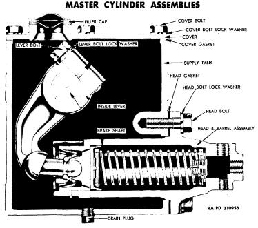
Figure 6 – Box Type Master Cylinder
